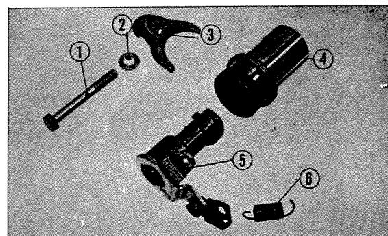
① Clutch adjuster locking bolt ② 6mm washer
