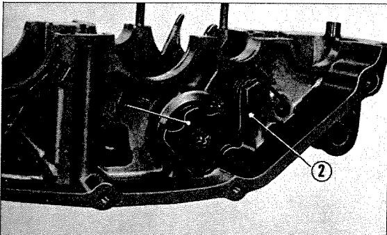
① Shift drum stopper plate ② Shift drum stopper
