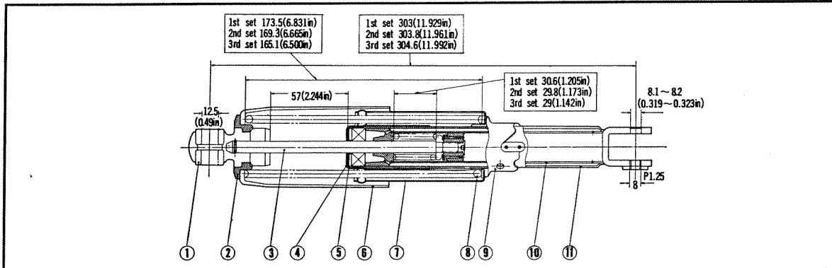
① Rear cushion upper rubber bush ② Rear cushion spring seat stopper ③ Rear damper piston rod complete ④ Staking
