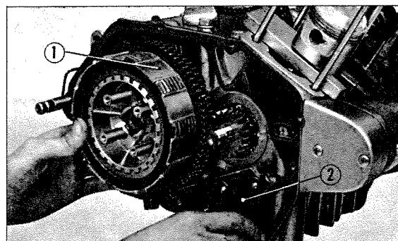
① Clutch outer ② Oil pump assembly
