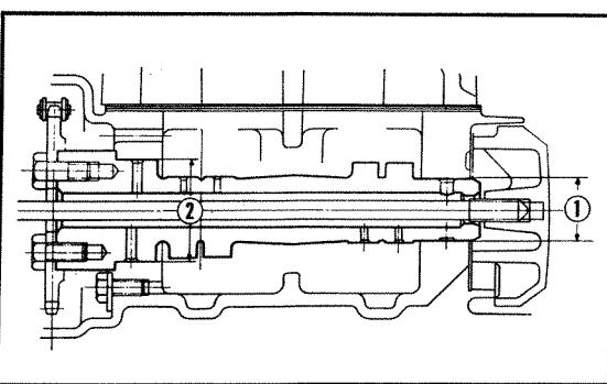
Fig. 3-147. Camshaft dimensions
