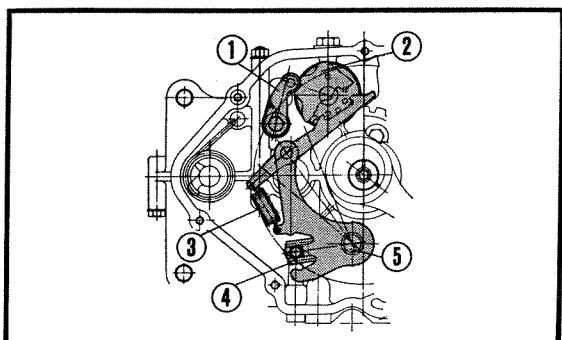
① Shift drum stopper ② Gear shift drum
