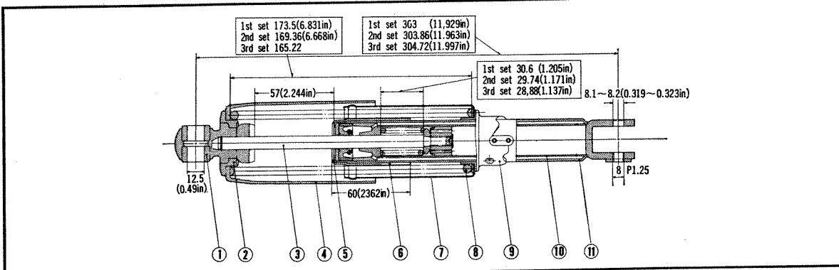
① Rear cushion upper rubber bushing ② Rear cushion spring seat stopper ③ Rear damper piston rod complete
