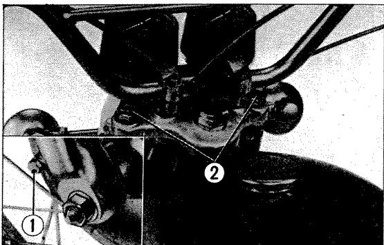
① Front fork drain plug ② Front fork top bolt
