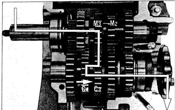
Fig. 9-48 C. 3rd gear (C<sub>4</sub> shifted)
