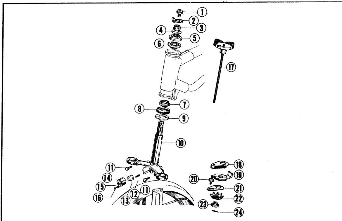
① Damper lock spring setting bolt ② Steering damper locking spring ③ Steering head stem nut ④ Steering stem washer
