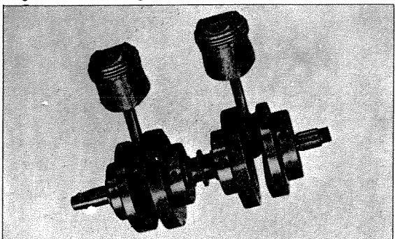
Fig. 3-73A. Crankshaft.
