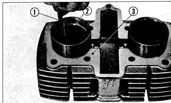
① Thickness gauge ② Piston ring ③ Cylinder
