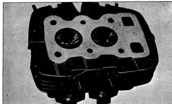
Fig. 3-136. Cylinder head
