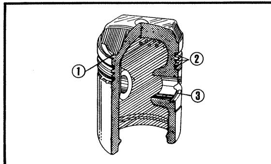
① Valve escape ② Piston ring grooves ③ Piston pin hole
