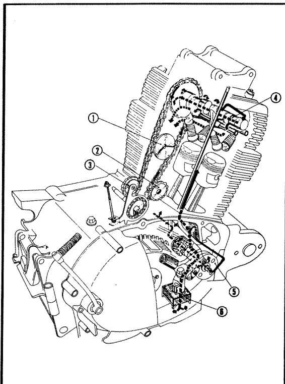
① Cam chain guide roller ② Cam chain idle roller
