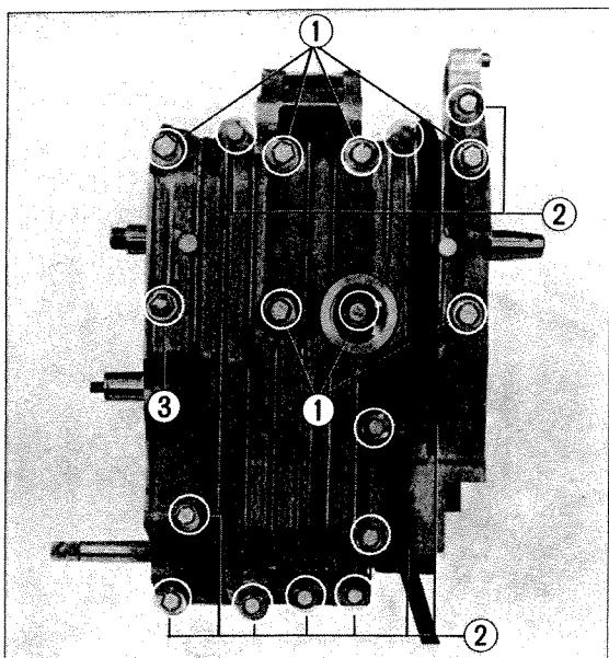
① 8 mm bolt ② 6 mm bolt ③ 8 mm cap nut
