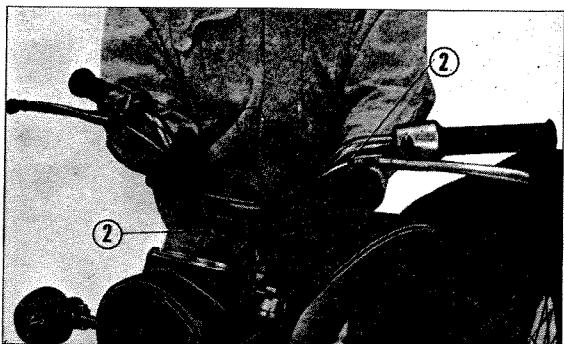
① Steering handle pipe ② Wire & cables
