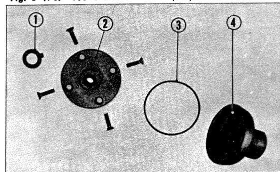
① Oil filter rotor washer ② Oil filter cap
