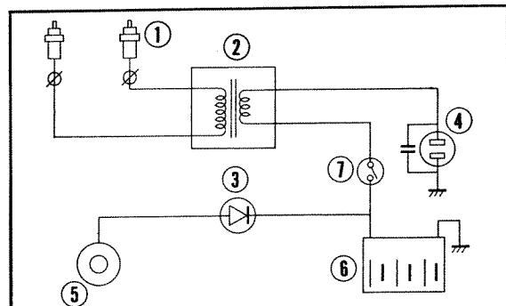
① Spark plug ② Ignition coil ③ Selenium rectifier
