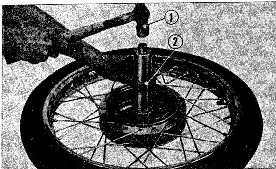
① Hammer ② Bearing installing tool
