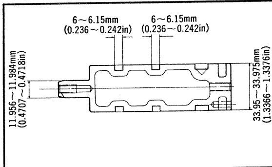
Fig. 3-193. Sectional view of gear shift drum
