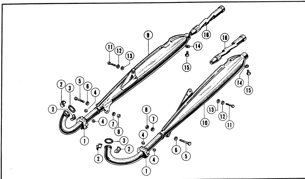
① Exhaust pipe joint   ② Exhaust pipe joint collar   ③ Exhaust pipe gasket   ④ 6 mm hex. nut   ⑤ 8×71 hex. bolt
