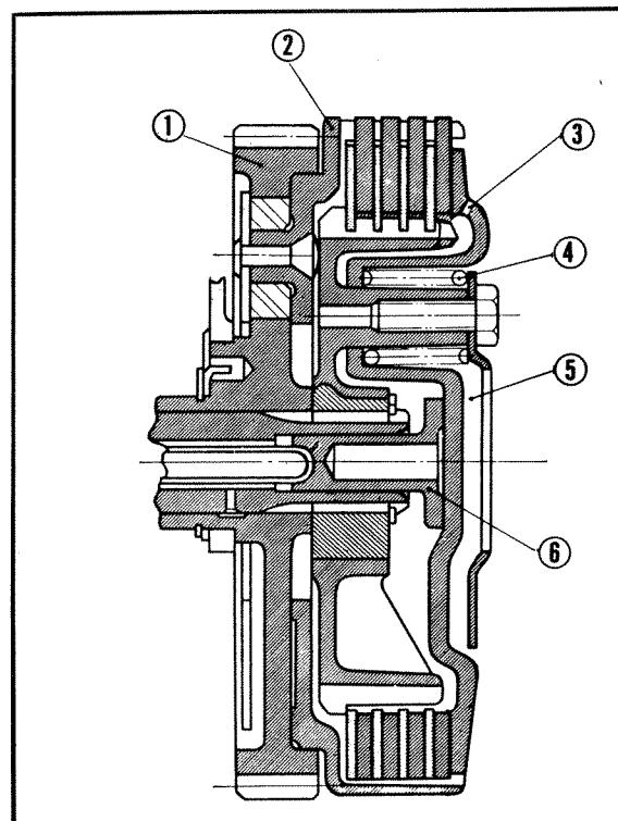
① Primary driven gear ② Clutch outer ③ Oil opening
