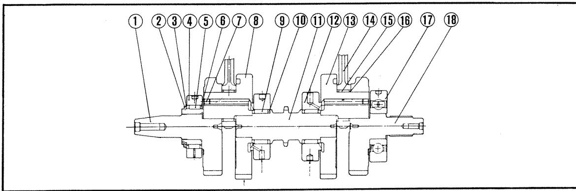
① Left crankshaft ② 35 mm circlip ③ 35 mm side washer ④ L. main bearing outer ring ⑤ 4×10 roller
