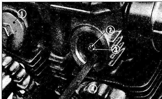
① Cylinder head cap ② Adjusting screw
