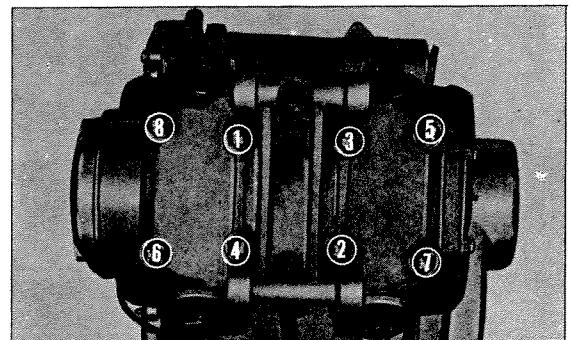
Fig. 3-16. Tightening sequence of the cylinder head
