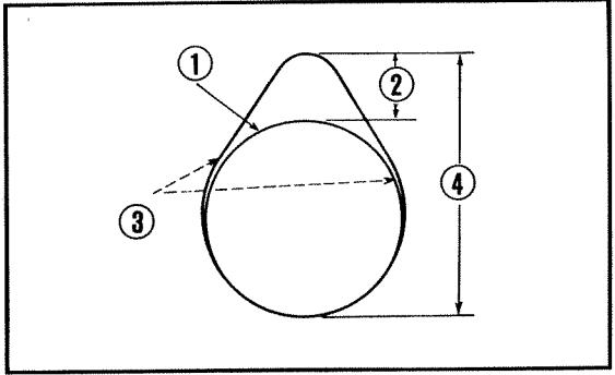
① Base circle ② Max cam lift ③ Buffer curve
