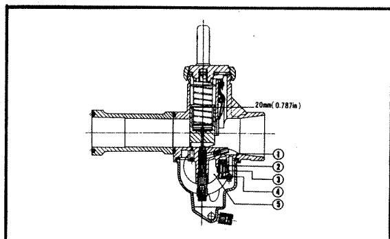
① Float chamber washer ② Float valve
