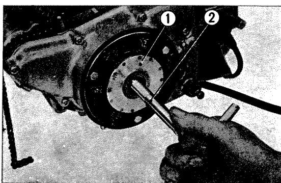
① Generator rotor ② Rotor puller
