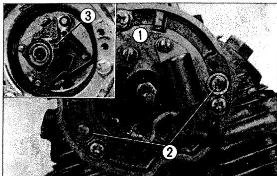
① Contact breaker assembly    ③ Spark advancer
