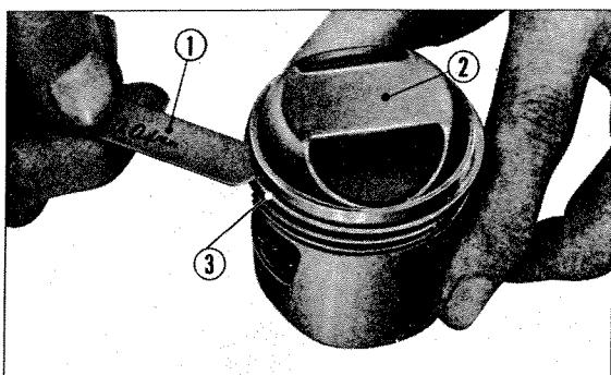
① Thickness gauge ② Piston ③ Piston ring
