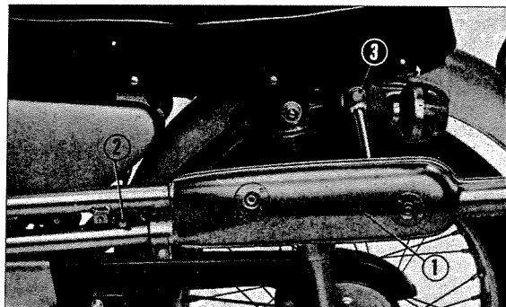
① Muffler ② Exhaust pipe setting bolt
