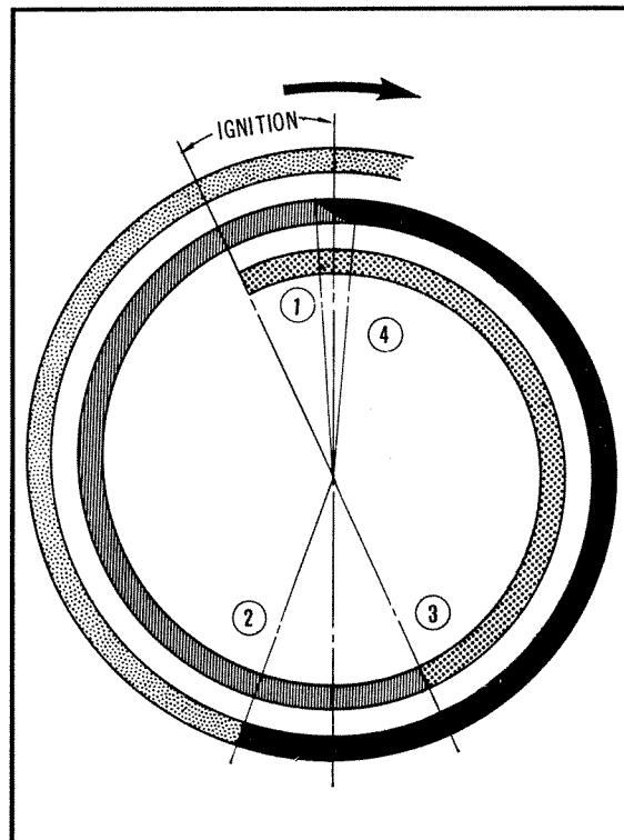
① Inlet valve opens 10° ② Inlet valve closes 40°
