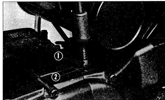
① Clutch adjusting bolt ② Locking nut
