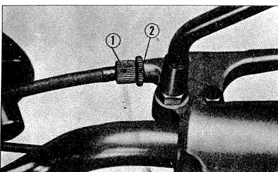
① Front brake upper adjuster ② Lock nut
