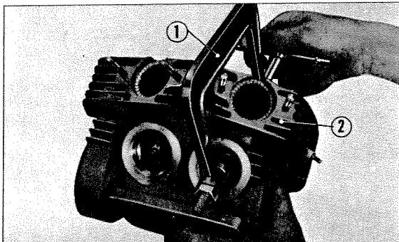
① Valve lifter ② Cylinder head
