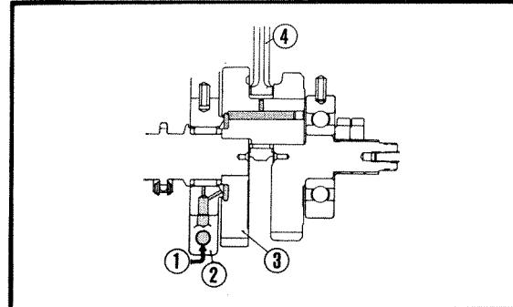
① Oil ② Center crank outer ring ③ Crank weight
