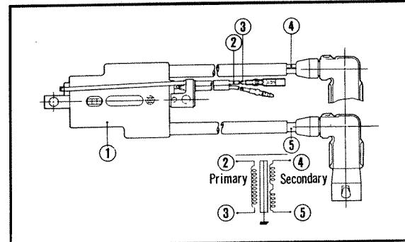
① Ignition coil ② Low tension lead
