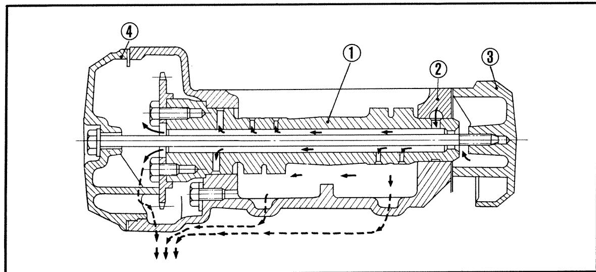
① Camshaft ② Cylinder head ③ Cylinder head right side cover ④ Cylinder head left side cover
