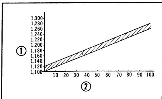
① Specific gravity (20°C) ② Residual capacity (%)
