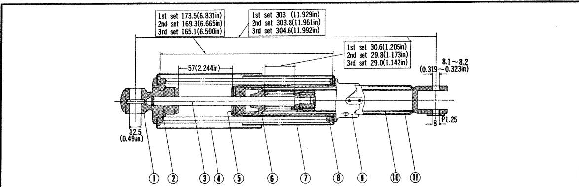
① Rear cushion upper rubber bush ② Rear cushion spring seat stopper ③ Rear damper piston rod complete
