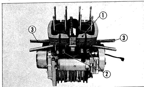
① Cylinder ② Piston base ③ Piston ring compressor
