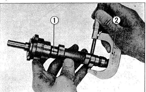
① Cam shaft ② Micrometer
