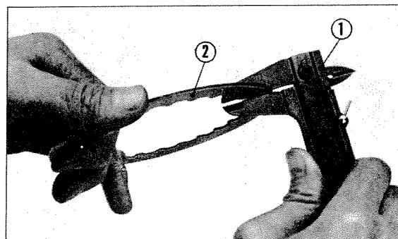
① Vernier calipers ② Clutch plate
