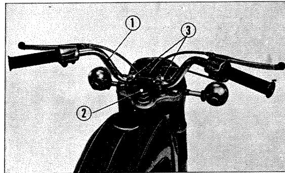
① Steering handle pipe    ② Steering damper knob
