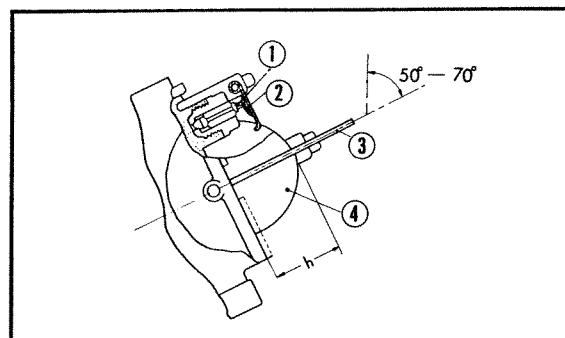
① Float valve ② Float arm ③ Float gauge ④ Float
