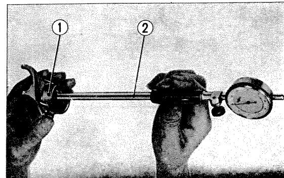
① Gear shift fork ② Cylinder gauge
