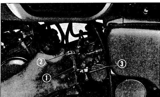
① Throttle cable    ② Carburetor cap    ③ Throttle valve
