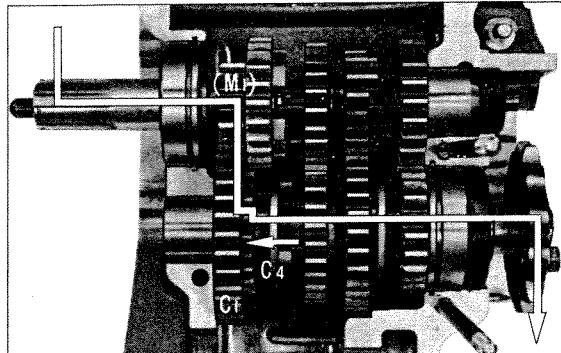
Fig. 9-48 A. 1st gear (C<sub>4</sub> shifted)
