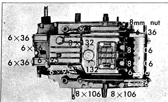
Fig. 3-71B. Bolts and nuts on the lower crankcase
