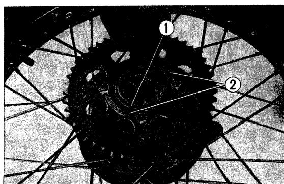
① Circlip ② 8 mm Special tongued washer
