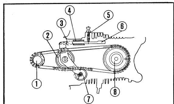
① Center crankshaft ② Cam chain guide roller
