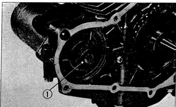
① Starting motor sprocket
