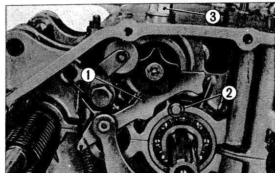
① Gear shift arm ② Projection ③ Neutral stopper bolt
