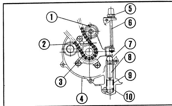
① Tensioner roller ② Tensioner arm ③ Timing sprocket
