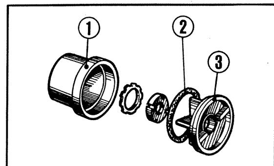
① Oil filter rotor ② 46X2 Oring ③ Oil filter cap
