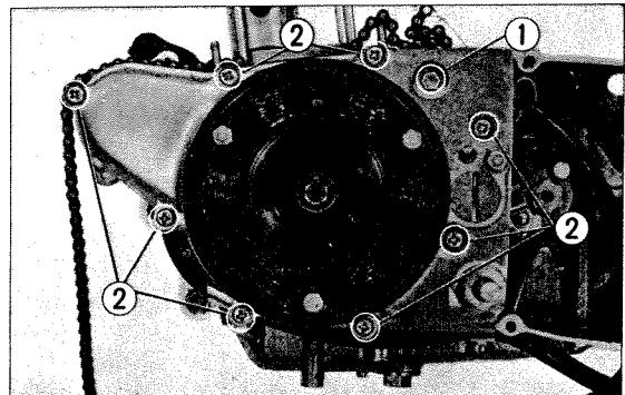
① Cam chain adjust ② 6 mm screw
