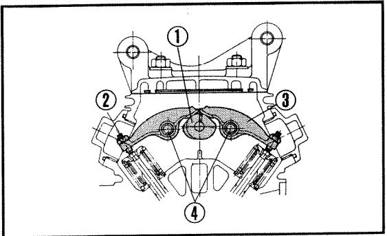
① Camshaft ② Tappet adjusting nut ③ Rocker arm
