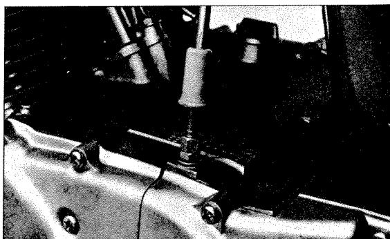
① Clutch cable lower adjuster ② Locking nut
