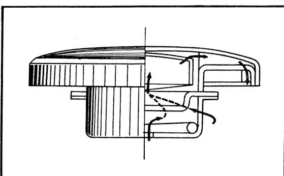
Fig. 6-11. Sectional view of the fuel tank cap
