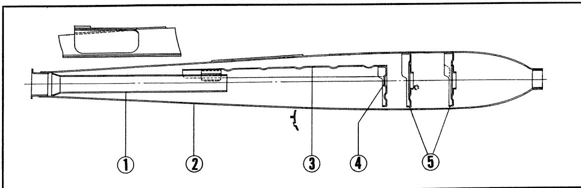
① Inner pipe   ② Muffler half   ③ Separator A   ④ Separator B   ⑤ Separator C
