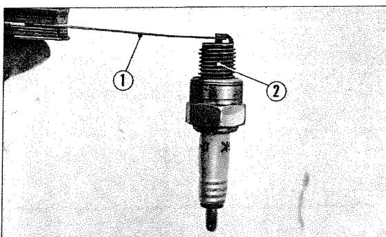
① Thickness gauge ② Spark plug
