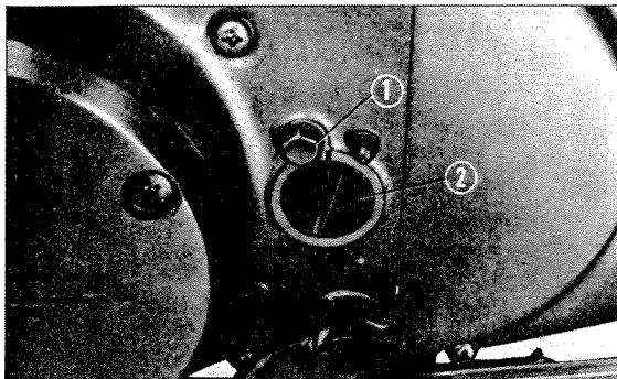
① Clutch adjuster locking bolt ② Clutch adjuster
