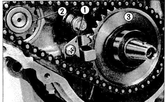
① Starting sprocket set plate ② Starting motor sprocket
