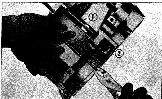
① Oil separator ② Oil separator set bar
