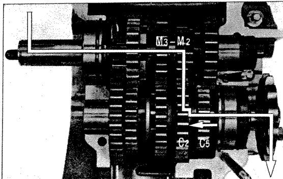
Fig. 9-48 B. 2nd gear (C<sub>5</sub> shifted)
