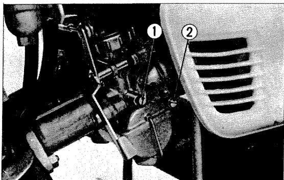
① Throttle stop screw ② Air screw
