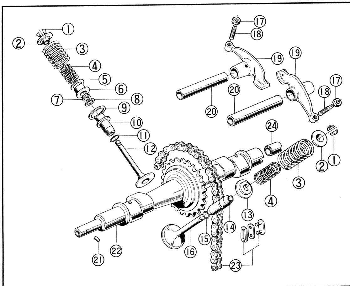
① Valve cotter ② Valve retainer ③ Outer valve spring ④ Inner valve spring ⑤ Inner seal ⑥ Valve stem seal cap
