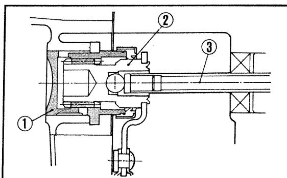
① Clutch adjuster ② Clutch lifter thread
