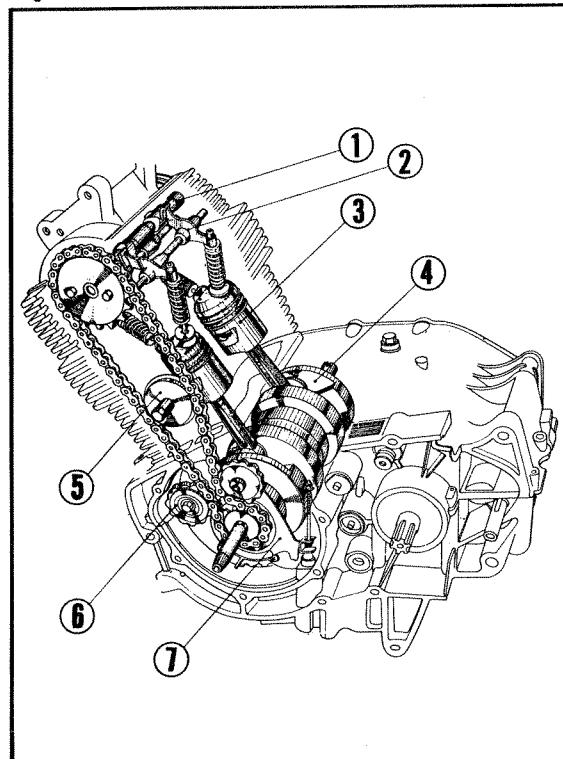
① Cam shaft ② Valve rocker arm ③ Piston
