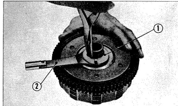
① 26 mm circlip ② Pump rod
