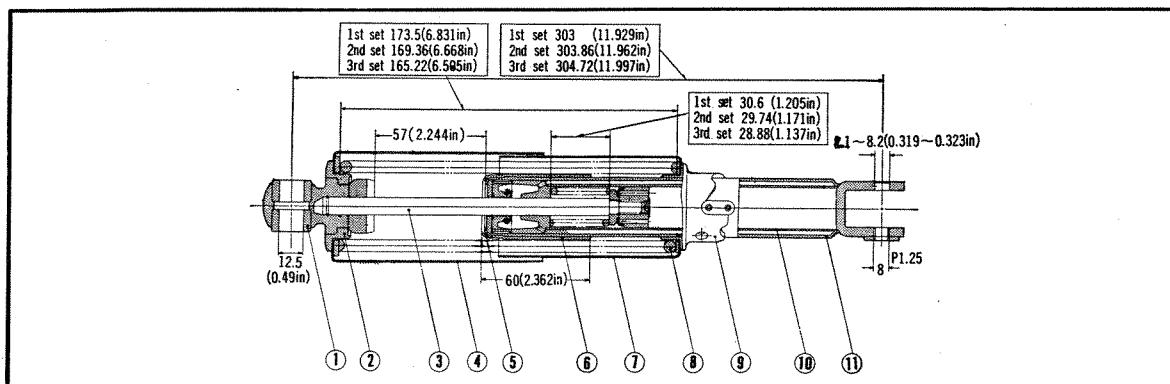
Fig. 4-49-4. Sectional view of rear cushion (CL175)
