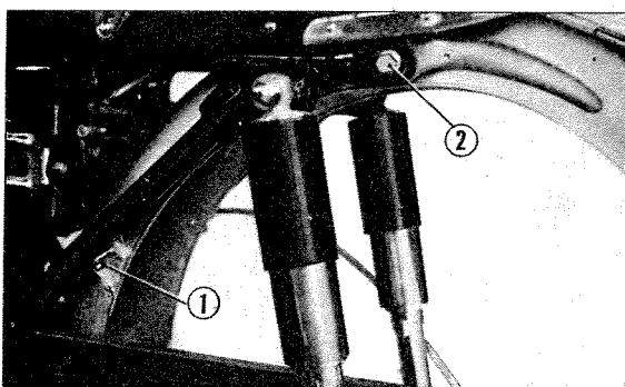
① 6×12 mm hex. bolt ② Rear fender setting bolt
