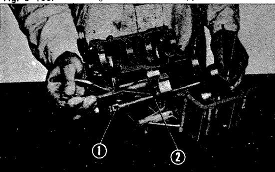
① Gear shift spindle ② 12 mm set ring
