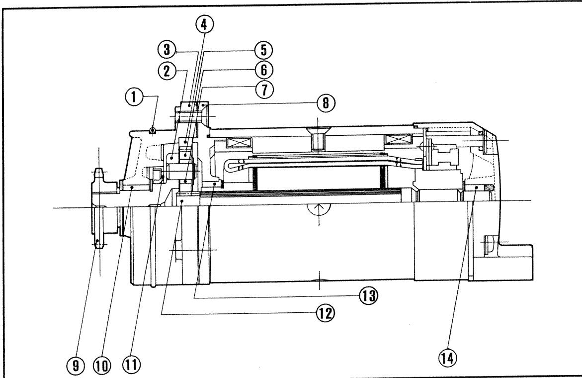
Fig. 5-22. Construction of starting motor
