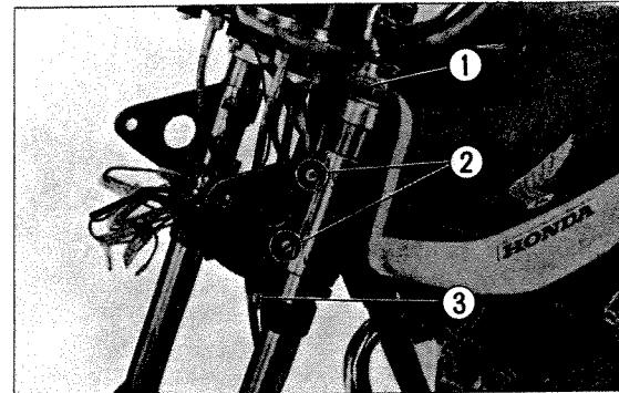
① Front for top bolt ② Headlight bracket setting bolt
