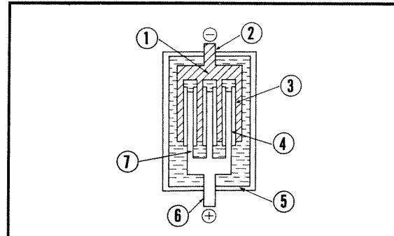
① Pole ②  $\ominus$  terminal ③ Negative plate ④ Separator & glass net ⑤ Container ⑥  $\oplus$  terminal ⑦ Positive plate
